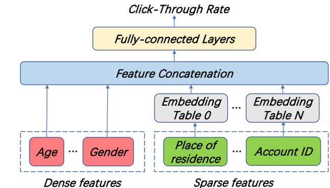
Fig. 1. High-level architecture of a typical deep recommendation model.
